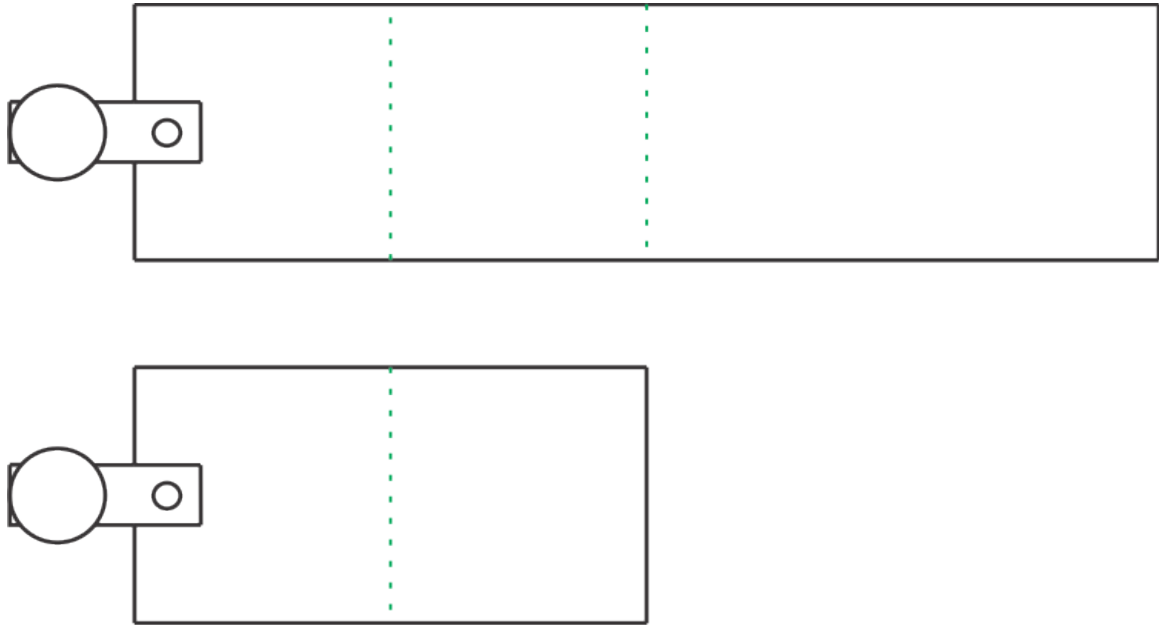
Figure 3.10: Top view of both aspect ratio plates showing the locations of chordwise laser planes by green dashed lines. The top part of the figure shows the two relative spanwise positions obtained for the \mathcal{R}4 plate while the bottom portion shows the single spanwise position acquired for the \mathcal{R}2 plate.
